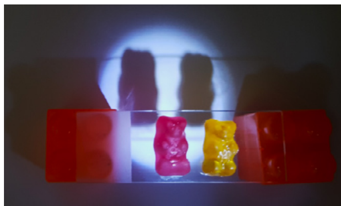
Figure 5: The shadows under red and yellow gummy bears when illuminated with white light
