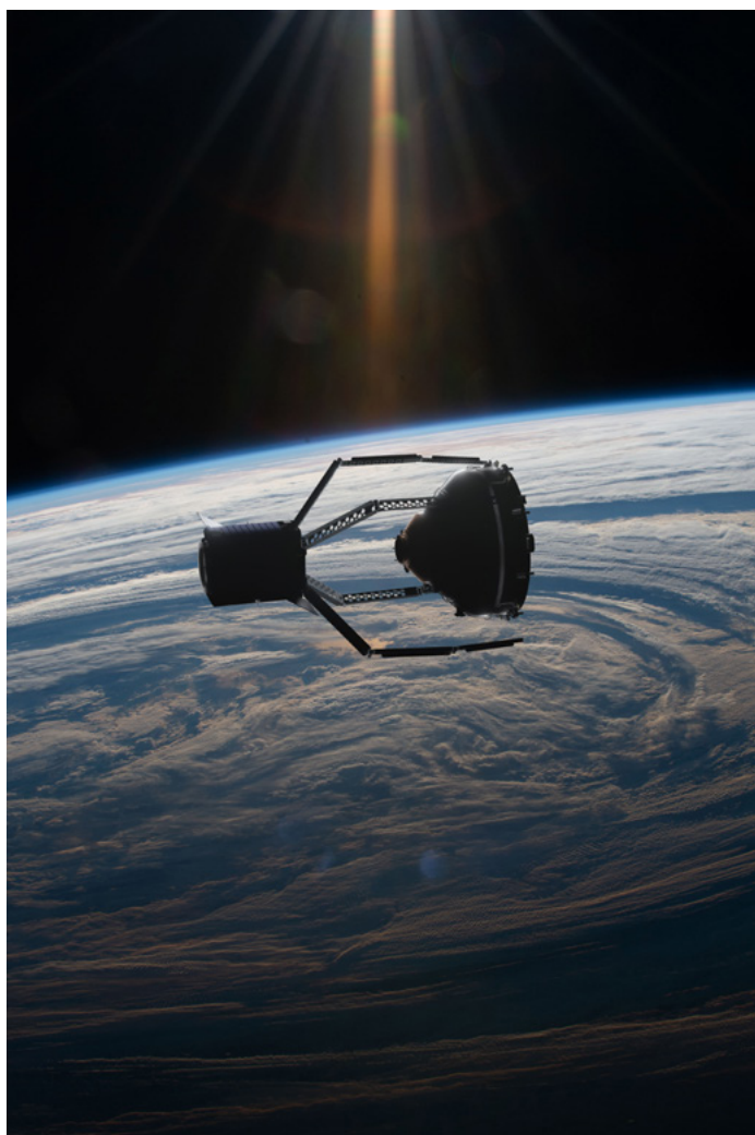
Figure 6: Artist's representation of the ClearSpace-1 mission to remove a Vespa upper stage using four robotic tentacles.
