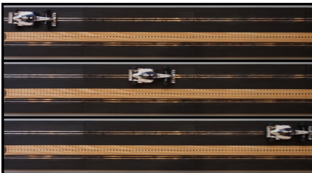
Figure 4: This is a repeat run for the toy car shown in figure 3, but, in this sequence, there are three usable frames, allowing acceleration to be investigated.
