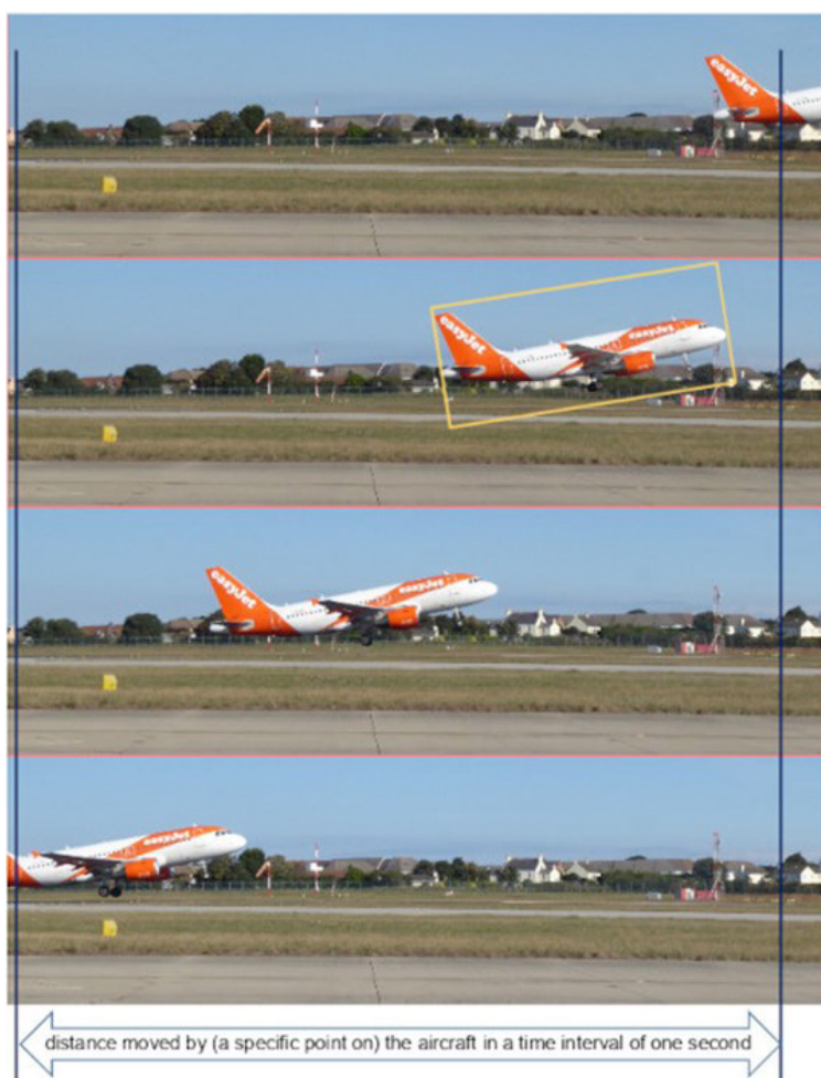
Figure 1: Composite of aircraft take-off sequence for Airbus A319-100 Image credits: Jon Tarrant, CC-BY-SA
