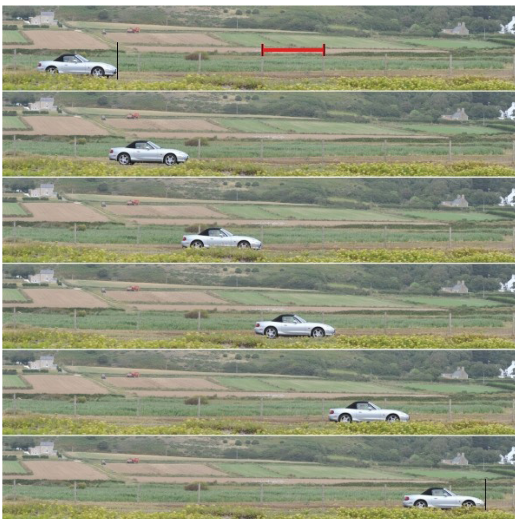
Figure 5: Road car photographed at 0.2 s intervals in front of fence posts spaced 3.4 m apart. See the the supporting material for a full analysis
