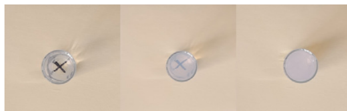
Figure 1: As the reaction of sodium thiosulfate and hydrochloric acid proceeds, the sulfur precipitate formed obscures a cross drawn under the vial.
