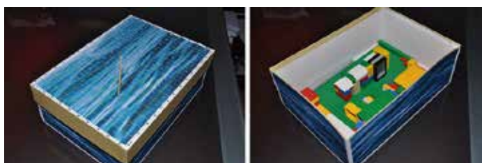
Left: The lid of the sounding box with a skewer probing the depth in a cell of the grid. Right: The mock seafloor in the sounding box
