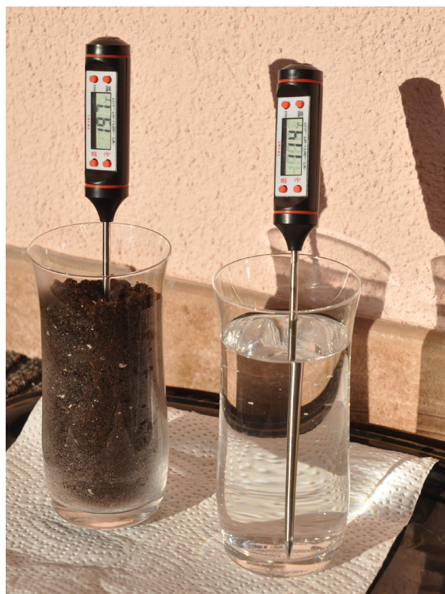
Equipment for testing the different heat capacities of water and soil
