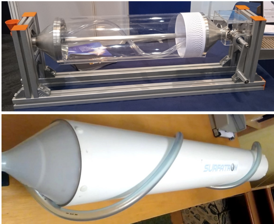
Figure 1. Top: Manually operated mechanical Surfatron built in a professional workshop, featuring stroboscopic lines for frequency calibration. Bottom: Home-made version Image courtesy of Ricardo Torres
