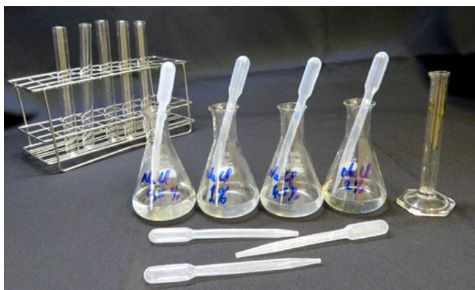
Test tubes, NaCl solutions, graduated cylinder, and pipettes Image courtesy of the authors
