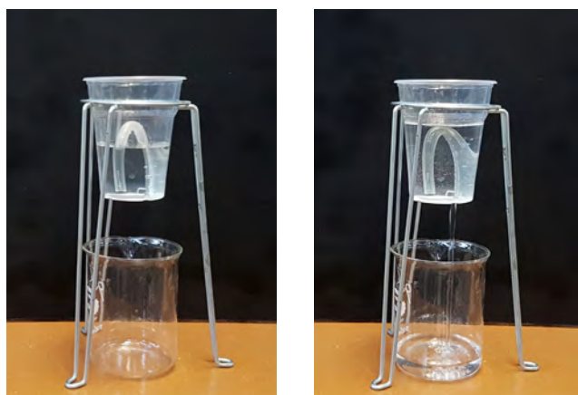
The Pythagoras' cup demonstrating the syphon principle Image courtesy of Panagiotis (Takis) Lazos
