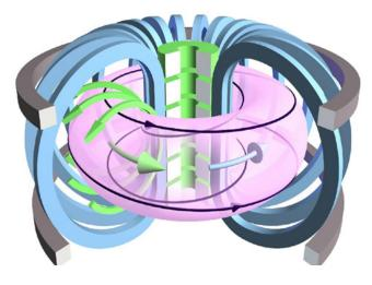
Schematic of a tokamak – the magnetic coils (shown in blue and grey) are used to control the fusion plasma (in pink) © UKAEA
