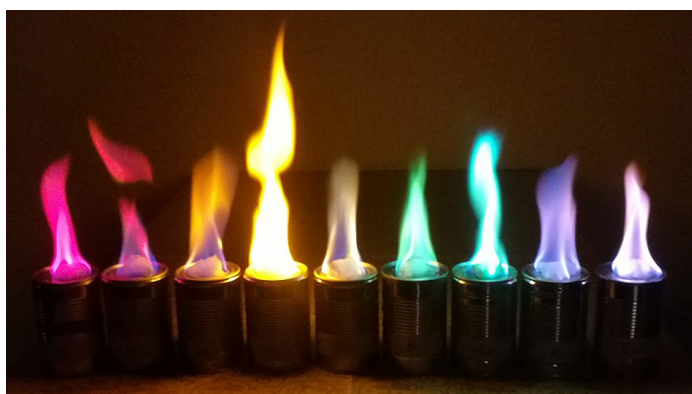
Coloured flames from methanol solutions of different compounds. From the left: lithium chloride, strontium chloride, calcium chloride, sodium chloride, barium chloride, trimethyl borate, copper chloride, caesium chloride and potassium chloride
