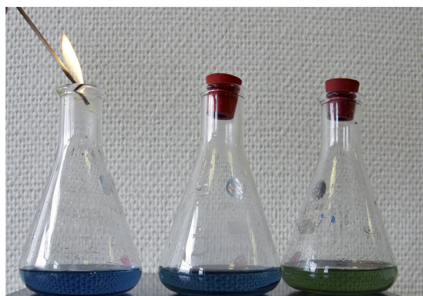
Figure 4: Experimental sequence: ignite the wooden stick; insert the stopper; note the pH after shaking the flask.
