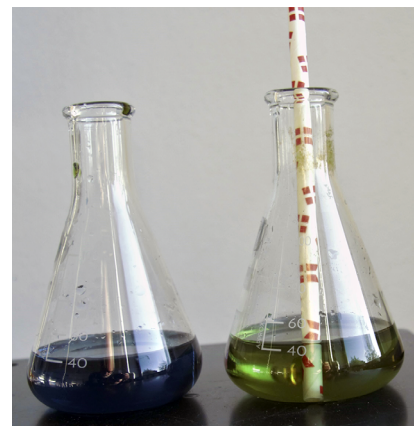
Figure 2: Fresh water and bromothymol blue indicator without (blue) and with (green) CO 2
