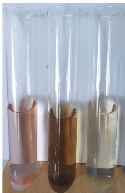
Figure 5: Hibiscus infusion before (left), and after adding sodium percarbonate (centre) and sodium dithionite (right) Marisa Prolongo
