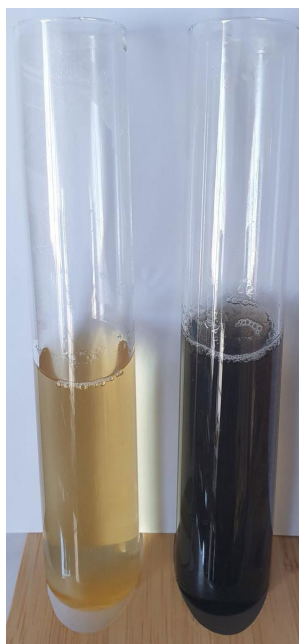
Figure 3: An infusion of black tea (left), and after adding a solution of iron(III) chloride (right)
