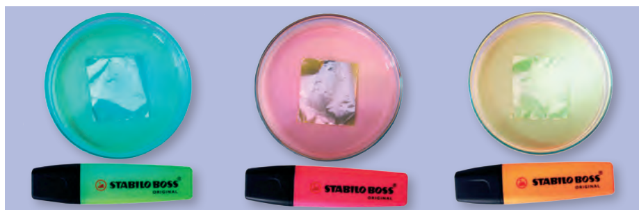
Figure 6: Superglue fingerprints on aluminium foil in highlighter solutions
