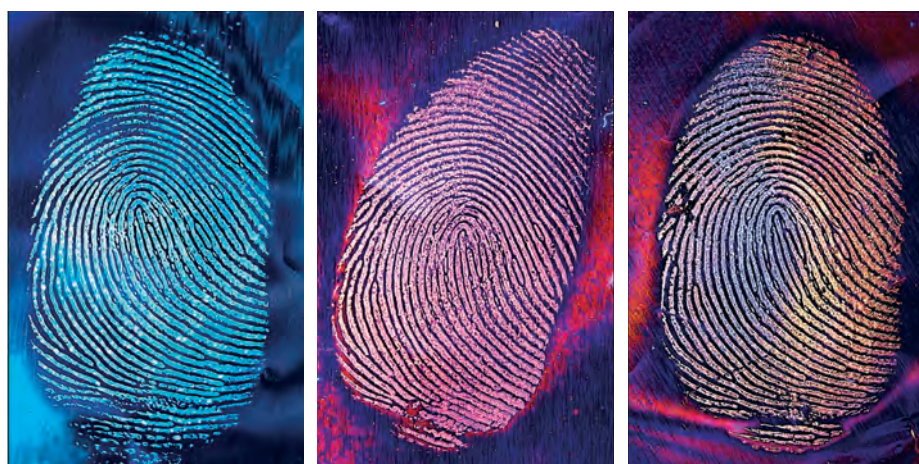
Figure 7: Fluorescent superglue fingerprints under UV light
