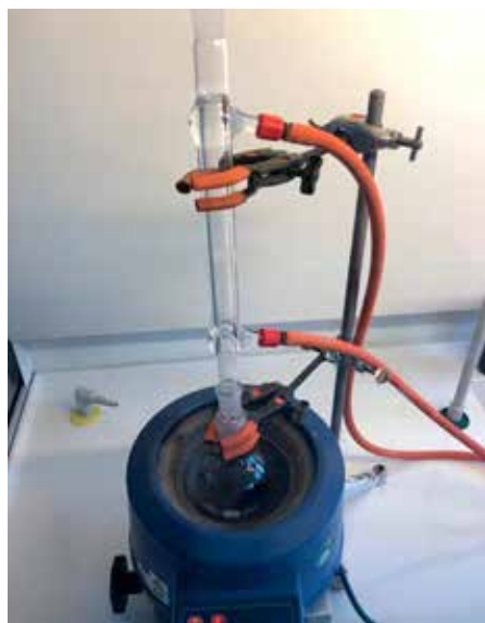
Flask, reflux condenser and heating mantle setup (steps 4–5)
