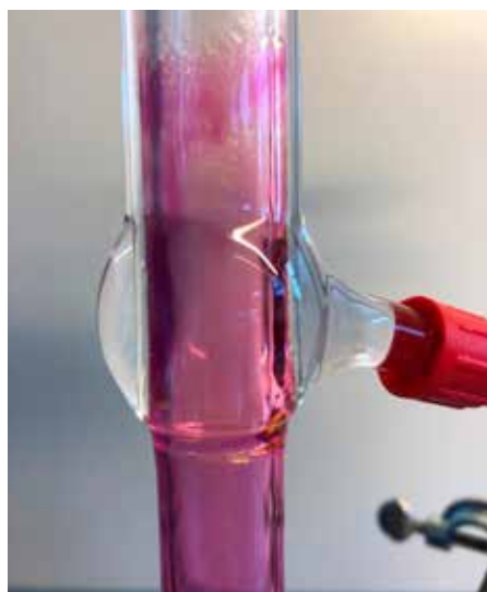
Iodine vapour in the reflux condenser
