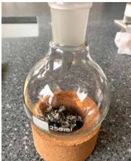
Tin and iodine in the flask (step 2)
