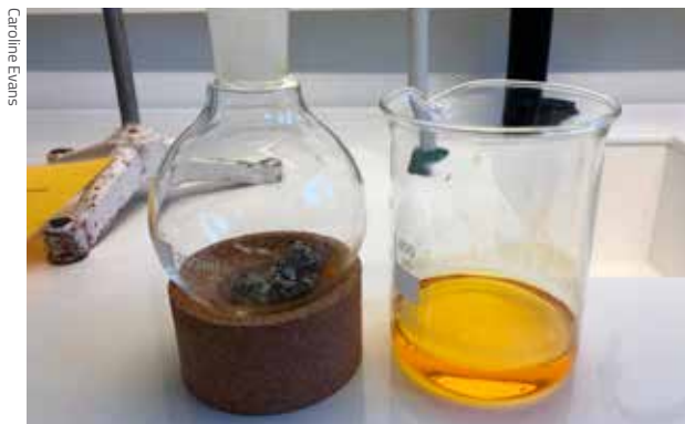
End of the reaction: orange liquid and residual tin (step 10)
