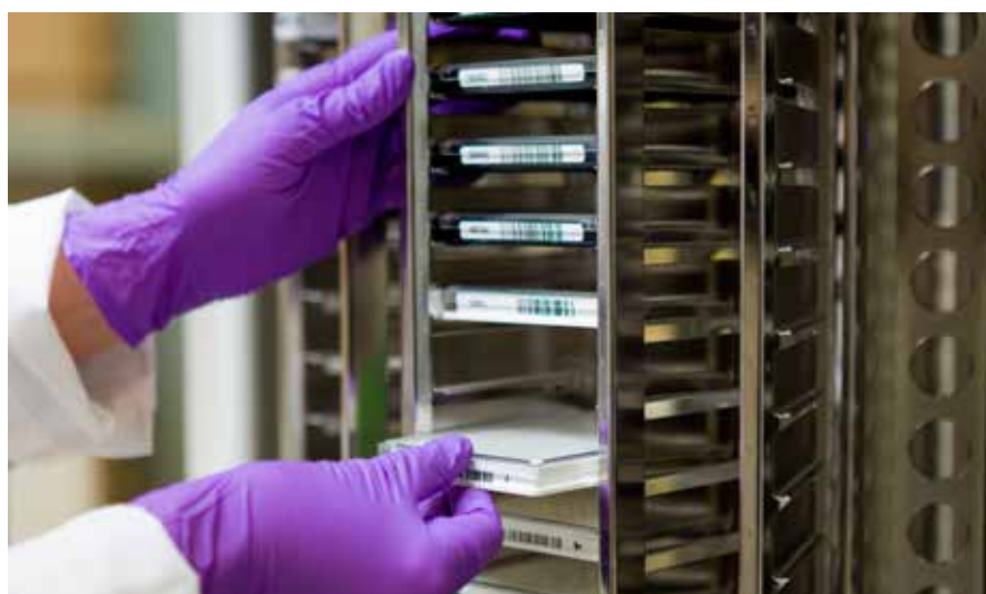
Plates are placed in a robot carousel to be rapidly tested using high-throughput screening.
