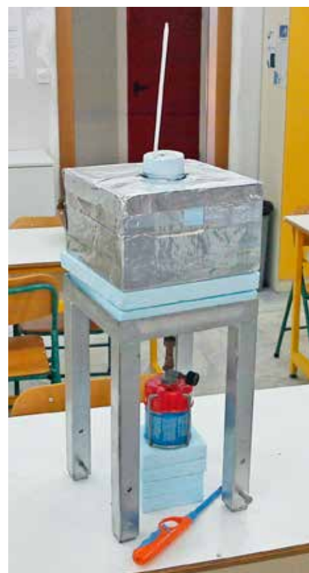
Figure 5: The finished calorimeter is ready for carrying out the experiments.
