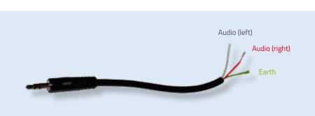
Figure 3: A stripped stereo audio cable shows two audio wires and one bare earth wire.
