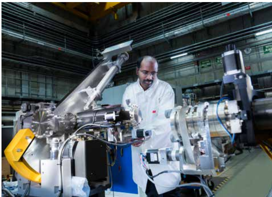
At European XFEL, a physicist works on the spectrometer used for monitoring the X-ray pulses fired at samples. The spectrometer has a beryllium 'window' for X-rays to reach the detectors.
