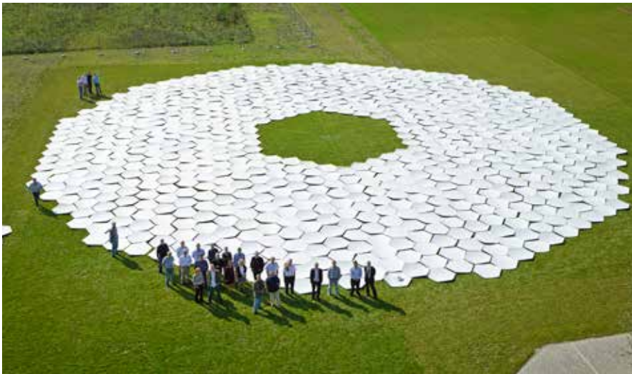
A scale mock-up of the ELT primary mirror, using cardboard versions of the mirror segments
