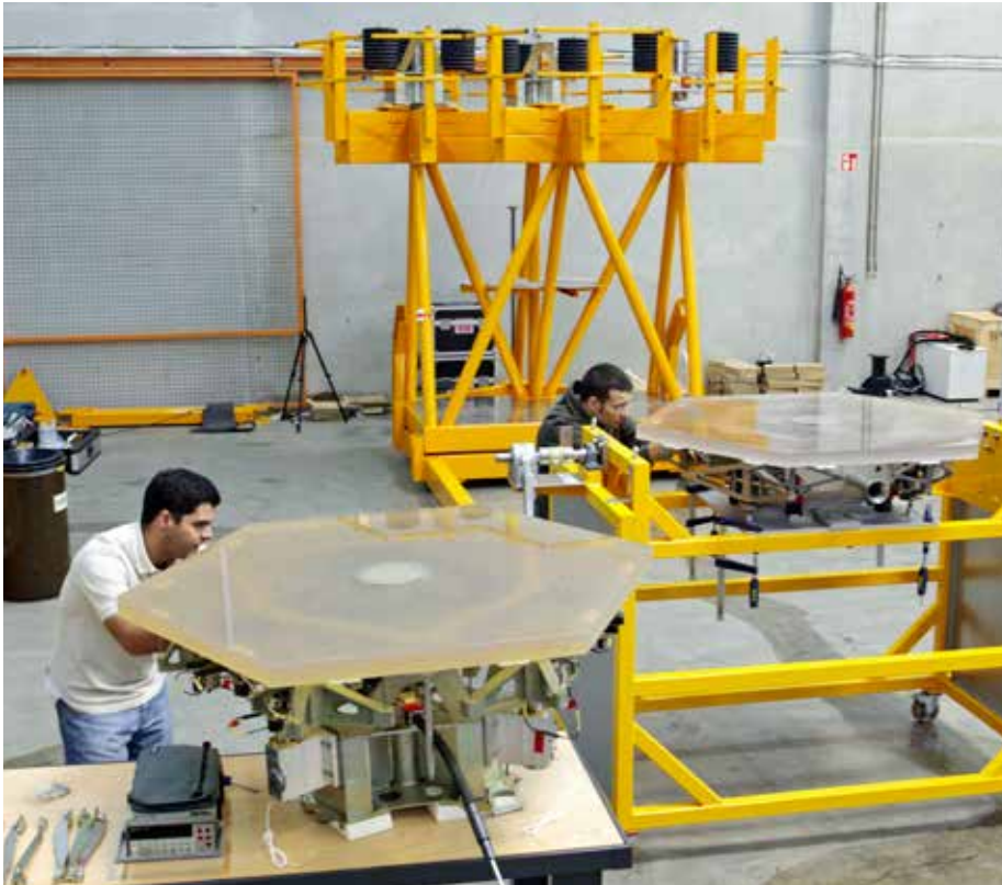
Testing of the sensors and actuators underneath two segments of the giant primary mirrors of the ELT
