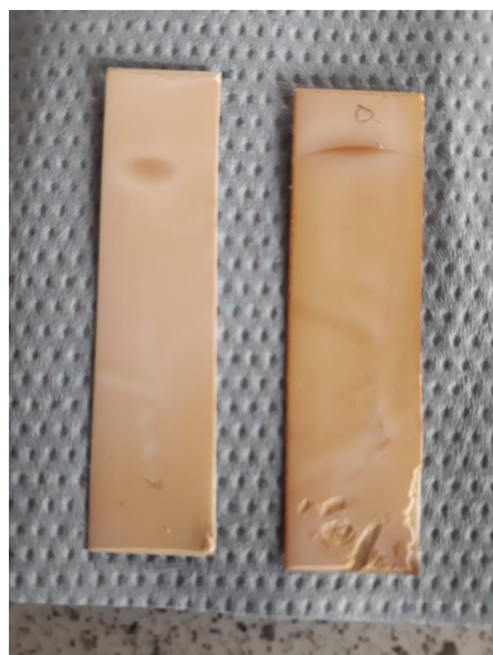
Figure 1: Thin layer chromatography plates with orange oil (left) and limonene (right) stained with permanganate
