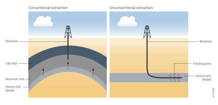
Figure 1: Comparison between conventional and unconventional gas extraction. In conventional extraction (left), gas moves upwards until it reaches an impermeable layer (cap rock). It collects within the reservoir rock, from where it is extracted by drilling. In unconventional extraction (right), the gas is extracted directly from the source rock, which must be fractured to obtain the gas. (Source: Hans-Martin Schulz, GFZ Potsdam)
