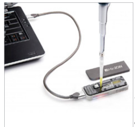
Figure 1: A nanopore sequencer connected to a laptop via USB. The DNA solution (yellow) is added with a pipette.
