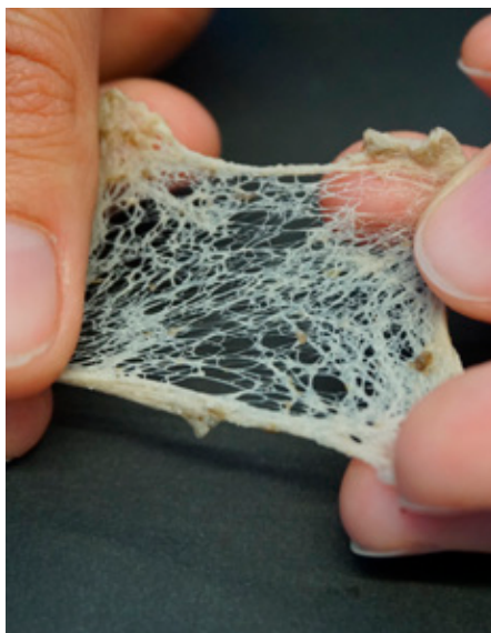
Figure 9: Gently pulling the net of rubber threads apart highlights the elastic properties of rubber.
