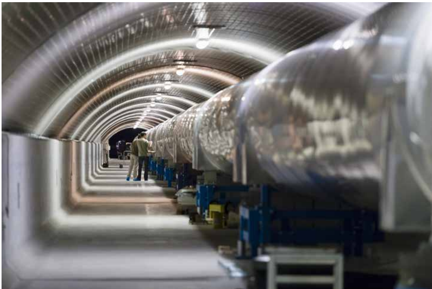
Figure 2: Inside one of Virgo's arm tunnels, showing the vacuum tube
