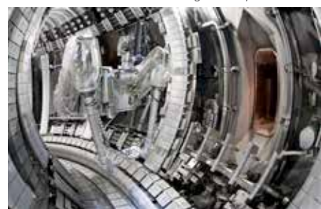
Interior view of the JET vacuum vessel with remote handling gripper
