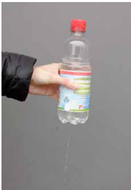
Figure 1: uncovering the hole in the cap: the water flows out through the hole in the bottom of the bottle.
