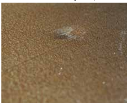
Figure 1: Close-up of a composite sample that has undergone impact damage. Note that the damage (which is a dent about 2 cm in diameter) looks quite minor.
