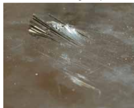
Figure 2: The reverse side of the same sample. Although not visible from the side that was impacted, the damage is catastrophic.
