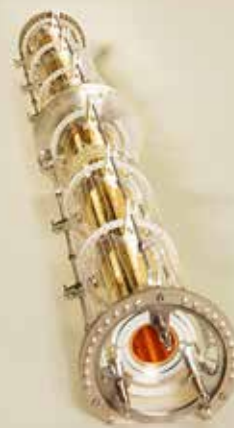
The inner part of the high precision mass spectrometer used in the research
