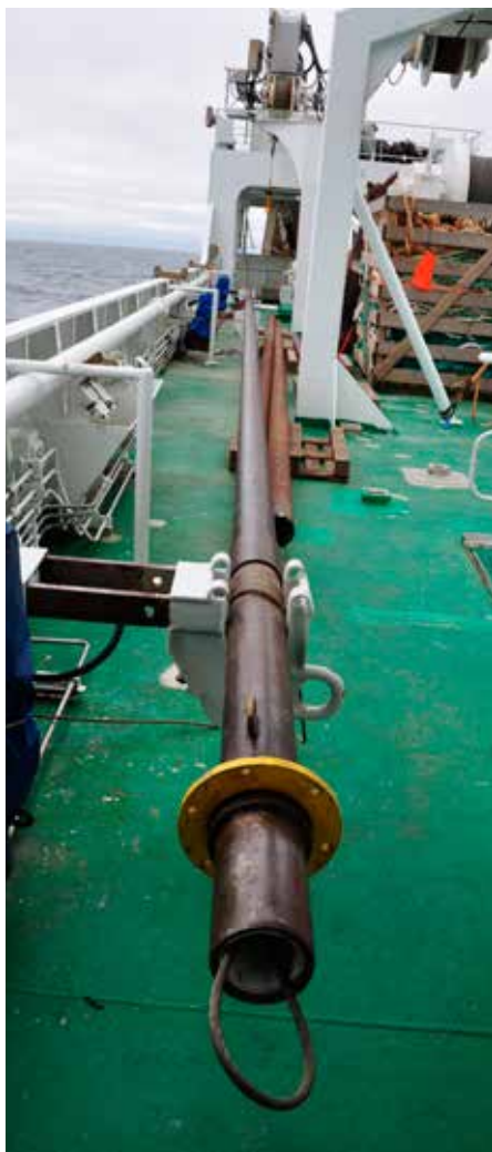
The calypso corer that took samples of the sea bed (left) required a huge machinery to be deployed (right). The cores collected were stored onboard the ship and carefully looked after by chief scientist Renata Lucchi (middle).
