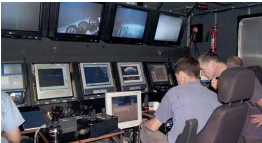
The inside of the ROV control van – the hub of activity during an ROV dive. Live feed from the ROV cameras can be seen on the upper monitors
