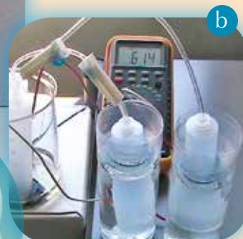
Figure 6: a) A system of chemical gas generator and gas holder; b) supplying the fuel cell with hydrogen and oxygen collected in gas holders
