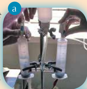
Figure 4: a) Opening the valves to allow the gases to pass to the electrodes of the fuel cell; b) electricity generation by the fuel cell
