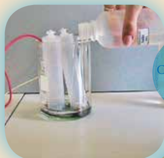
Figure 3: Demonstration of the stoichiometry of the water decomposition
