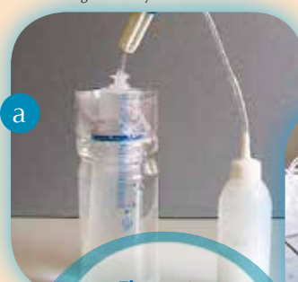
Figure 6: a) A system of chemical gas generator and gas holder; b) supplying the fuel cell with hydrogen and oxygen collected in gas holders
