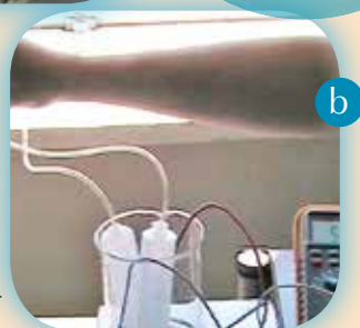
Figure 4: a) Opening the valves to allow the gases to pass to the electrodes of the fuel cell; b) electricity generation by the fuel cell
