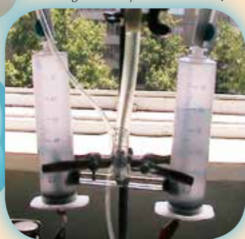
Figure 3: Demonstration of the stoichiometry of the water decomposition
