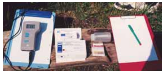
Testing the water samples – in both the field and the lab. A range of equipment was used, from pH strips to datalogging sensors
