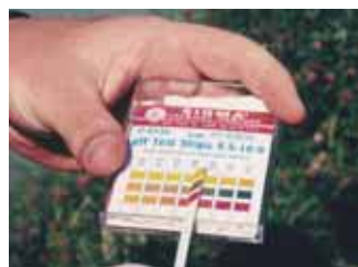
Testing the water samples – in both the field and the lab. A range of equipment was used, from pH strips to datalogging sensors
