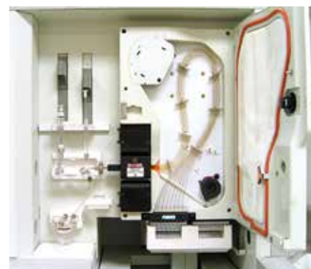
A DNA sequencer, showing the capillary array and blocks and syringes.
