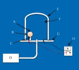
**Figure 2**: The experimental setup for activity 1. Inside the vacuum chamber, the sphere lies on an aluminium support. A magnet is placed inside the sphere, forming one electrode, and the second electrode is suspended from the top of the vacuum chamber.
