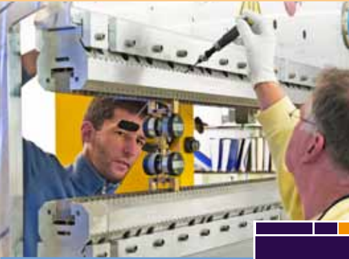
Tuning the pole heights of an undulator in the magnetic measurement laboratory.
