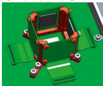
The LUCID detector designed by the Langton school
