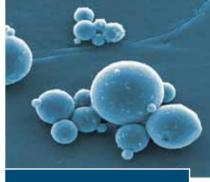
Fly ash particles as seen under a scanning electron microscope
