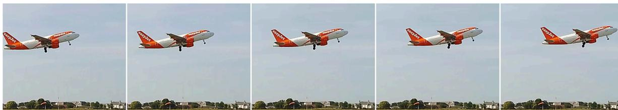
Sequence 1: Alternate frames extracted from a nine-frame sequence when the whole of the aircraft was in full view. The interval between each of the images shown here is 1/15 s, giving a total time of 4/15 s.
