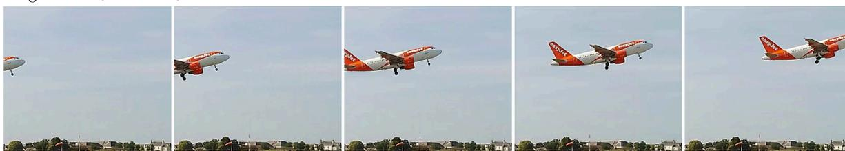
Sequence 2: In this sequence, every sixth frame has been extracted from the maximum time when a single feature (the nose wheel) remained in view. The interval between each image shown here is 1/5 s and the total time for the full 25-frame sequence is 4/5 s.
